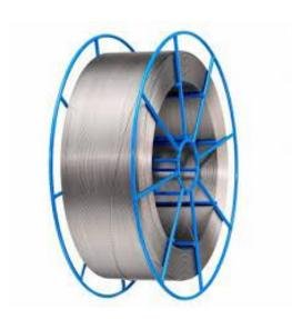
Panda Weld manufactures clean & layer wound wire for submerged arc welding from 1.60 mm (0.0625") to 5.00 mm (0.1875") in various grades in bright as well as in matte finish. The tensile strength, helix and cast diameter is engineered to precise tolerance: to ensure perfect "Pay-Off".
